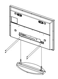
Two or more people should carry the PDP. Never lay the PDP on the floor because of possible damage to the screen. Always store the PDP upright.
